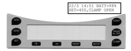
On the upper row date and time are shown together with the remaining battery capacity in %. The lower row shows the set collection volume and the tube clamp position.
