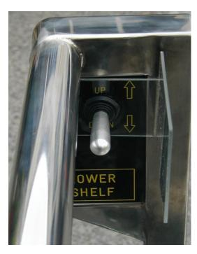
Pulling up or pushing down the levers directly below the cart handle opens the CO2 gas line and thereby moves the shelves. (See "Operating the Adjustable Shelves").
