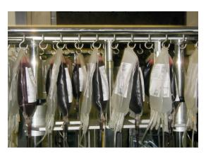
With the upper shelf down & the lower shelf up, both positioned at the operator's most comfortable working position, place the blood bag sets on the hooks, evenly distributed around the cart. There are 48 hooks and any number up to the maximum load of 48 filled bags or 79lb (36 kg) weight can be loaded. Do not lift more than 36kg at one time separately on either shelf. Place the receptacle bags to receive the Leuko-reduced blood, on the lower shelf. The shelf is designed to have the bags
