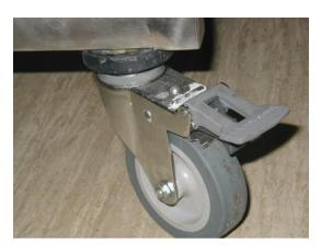
Four swing and lock high strength chromed caster wheels provide for easy rolling. They also contain a brake to lock the cart in position. Always lock the wheels when the cart is left unattended. The locks are activated by pushing the foot down on the lever that is located at the front edge of each wheel. To unlock, lift the foot up under the protruding lever or push the foot down on the top button until the lock clicks off.
