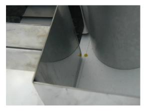
The Lower Shelf is made in two halves for easy cleaning & removal. To dismantle the lower shelf, remove the metal retaining bars at both ends of the assembled shelf, pull the two halves apart & remove each shelf from the frame. When re-assembling, locate the guide bars underneath each shelf half by lining up each shelf half with the yellow locating spot on the frame. Push forward until the shelves are fully back into position. Replace the metal retaining bars.
