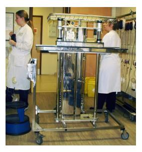
The two shelves are raised & lowered by two levers, each located underneath the handle, one lever for each shelf. (See "Operating the shelf levers").
