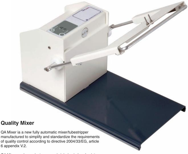
QA Mixer works against ergonomic injuries in hand wrists and shoulders which happens during manual operation. QA Mixer strips the tube and mix the bag automatically. QA Mixer is adjustable from 3-10 stripping cycles and 3-10 mixing cycles. For example the tube will be stripped 5 times and the bag will be mixed 10 times between each strip. QA Mixer is suitable for all blood bags on the market.
